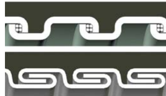
Square-Locked Design with cord packing 3/8" - 1-1/4"
